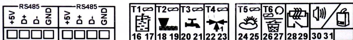
Fig. 9. Description of the sensors terminal strip.
