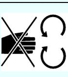
The transport worm may start operating without warning. Switch off power supply before lifting the cover.
