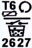
*Fig.26. Identification of the fuel level sensor connecting terminals.*
