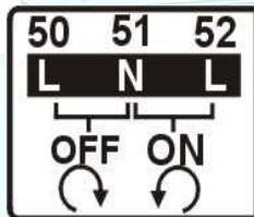
The mixing valve actuator shall be connected to the terminal strip (8) (fig. 7) terminals identified with the symbol shown on figure 19. The protective wire shall be connected to a terminal of the PE terminal strip (9) (fig. 7). The recommended cross-section of the actuator's connecting cable is stated in table 1.
