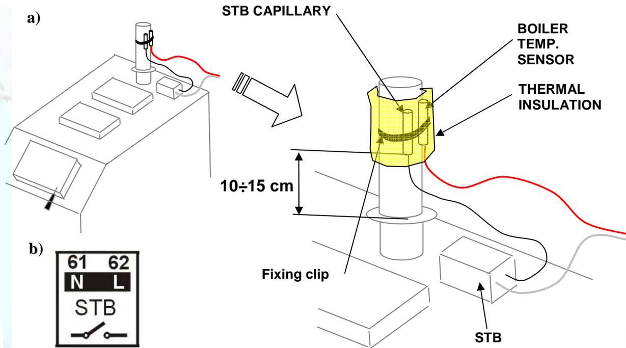
Fig.15. a) STB installation, b) identification of controller terminals
