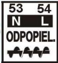
The cable used to connect the ash removal system motor shall have the cross-section specified in table 1. Ash-removal motor winding shall be connected according to the diagram located inside the connection box.
