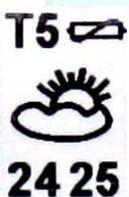
*Fig.25. Identification of weather sensor connecting terminals .*
