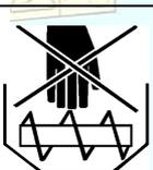
The device may periodically switch on without warning. Do not perform any works on a connected and switched on device.
